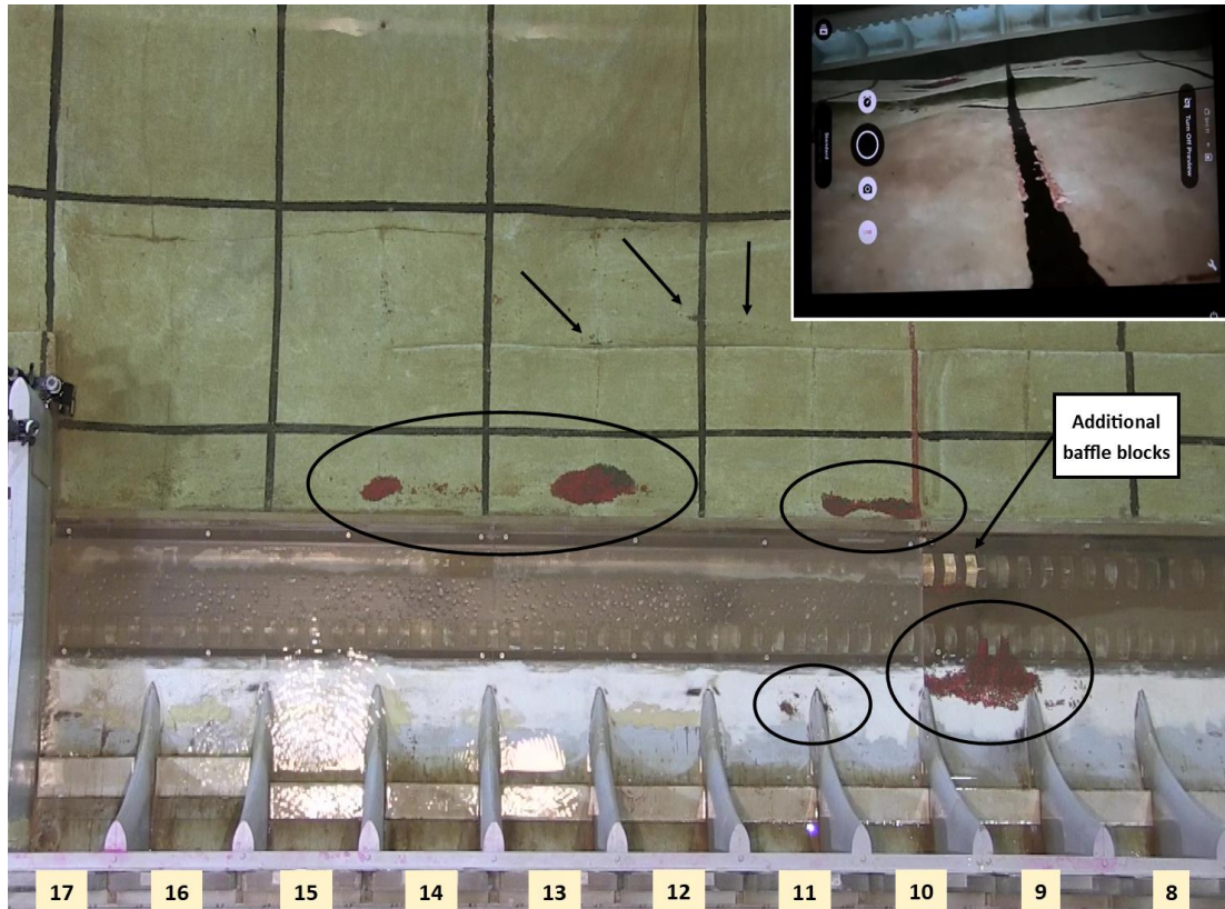
Figure 3-12. Final rock positions at the conclusion of test 5.
